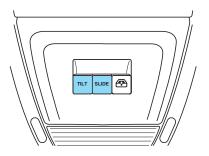
**Bounce-back:** When an obstacle has been detected in the moon roof opening as the moon roof is closing, the moon roof will automatically open and stop at a prescribed position.
